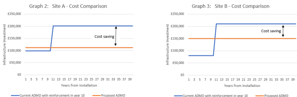
Graphs 2 and 3; Cost comparison for two sample developments with the revised ADMD applied against current design methodology with reinforcement works undertaken in year 10.
